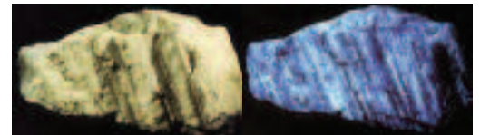
Fig 6: Strata-bound deposit at Mittersill/Austria Quartzite with rich scheelite at Ostfeld (open pit mining); daylight illumination (left) and UV illumination (right); note the stratiform grain sequence.
