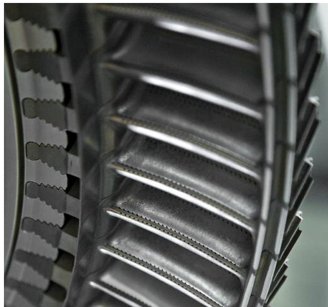
Figure 16: Showing turbines blades attached to a disc rim. © Rolls-Royce plc
